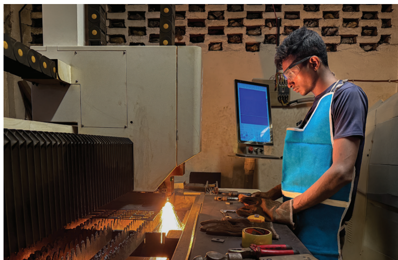
Metal sheets are being precisely cut with the help of a Computer Numerical Control laser cutting machine.
